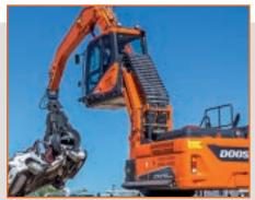
Hydraulic Elevating Cab (DX210WMH-5 – Standard) (DX225MH-5, DX300MH-5 – Option) With increased hydraulically controlled variable cab height, you can set your vantage point for an optimal view of your attachment and work area, allowing for maximum productivity.
