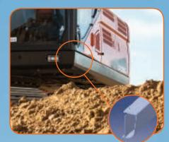
**D-Channel Frame Design** This innovative upper-structure frame design adds strength to withstand more side shock and protect vital machine components.
