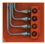
**Centralized Arm and Boom Grease Points** Daily maintenance is critical – and it's simple with the centralized grease banks on the arm and base of the boom.
