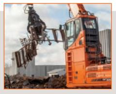
Fixed Cab Riser (DX225MH-5, DX300MH-5) The standard, fixed cab riser provides an excellent view of your attachment and work area for maximum productivity. The cab and riser can be hydraulically lowered for transport.
